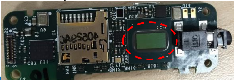
The Testchip Form Factor Test Board
